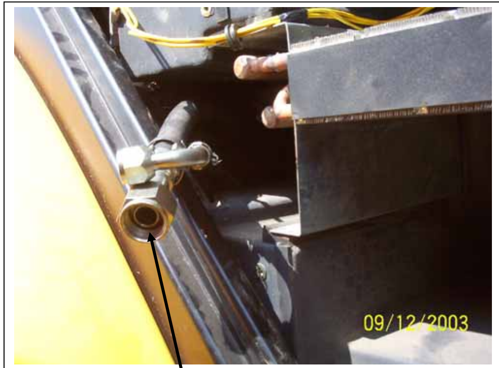
A/C hoses coming up with heater hoses into the cab
