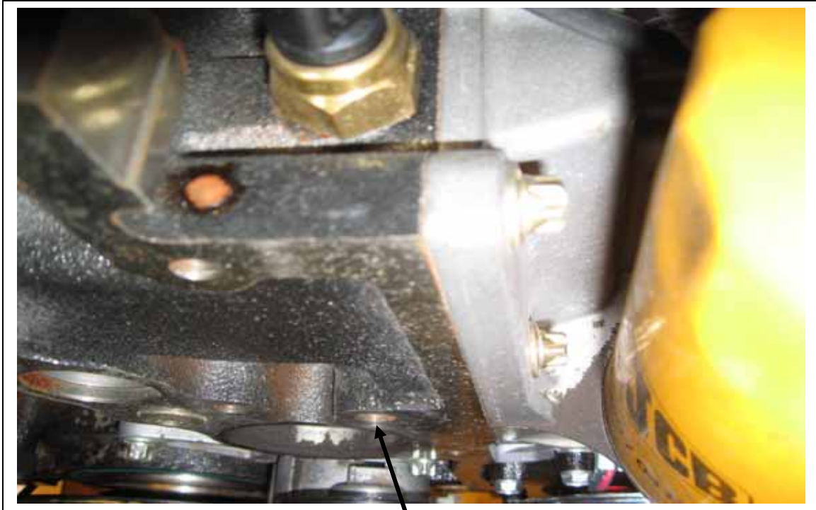
Mount the back side idler pulley in this M10 threaded hole.
