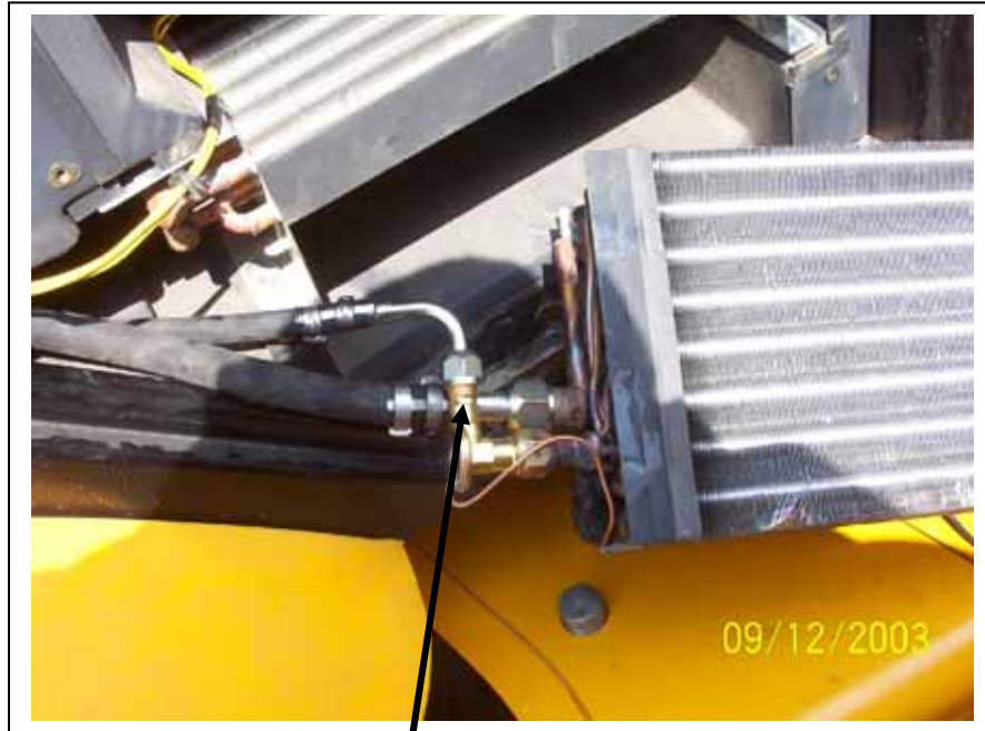
Connect the A/C hoses to the evaporator before sliding into place
